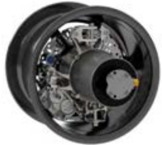
In-wheel Motor - First Design
